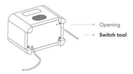
The power switch is located under the clock to prevent easy access in the mornings. To use the switch, you'll need the **switch tool** from the Defuse Panel. Simply poke the tool into the opening until the switch clicks on or off.
