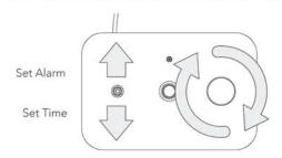
Push and hold the **toggle switch** up or down to set the time or alarm. A green backlight indicates PM time. Spin the **wheel** to change the time, and press it to switch between hours and minutes. Once you're done, release the switch to set.
